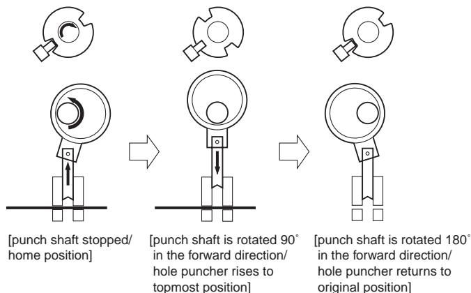
2) A hole is punched in the trailing edge of the second sheet.
