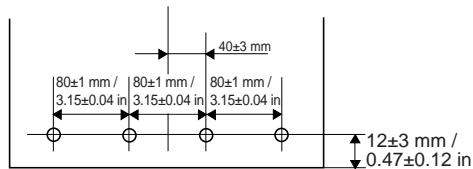
[4] Puncher unit-P1 (4-Hole (SWD))
