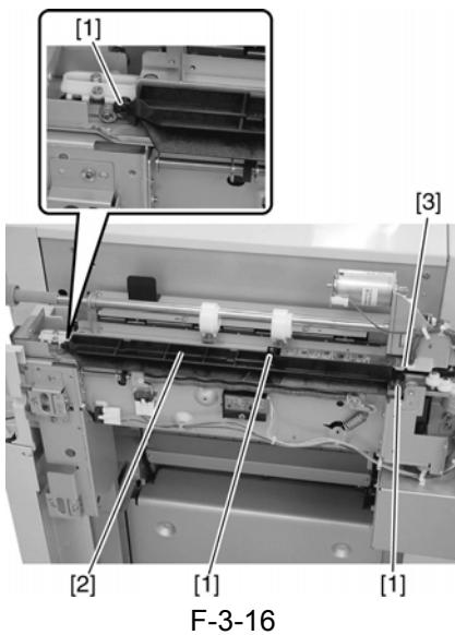
4) Disconnect the connector [1] and remove the screw [2], and remove the horizontal registration home position sensor [3].
