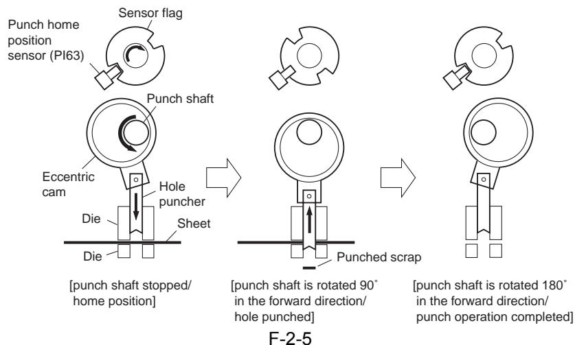
When two holes are punched, the 3-hole puncher is fed reciprocally in the escape direction (hole puncher rise direction) as shown below.
