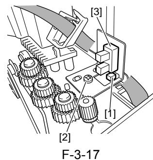
5) Turn the gear [1] in the direction of the arrow, and move the punch unit section [2] to the far side.
