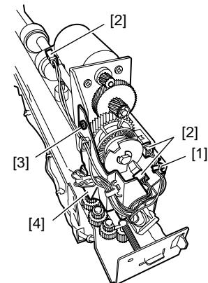
8) Lift up the front side of the punch unit section [1] first, then move in the direction of the arrow to remove the punch unit section [1].
