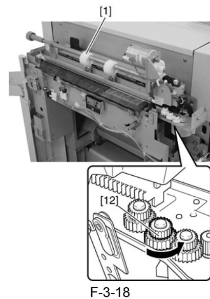
6) Remove the tie wrap with lock [1] while holding its claw between your fingers. (The tie wrap must be removed without being cut.)
